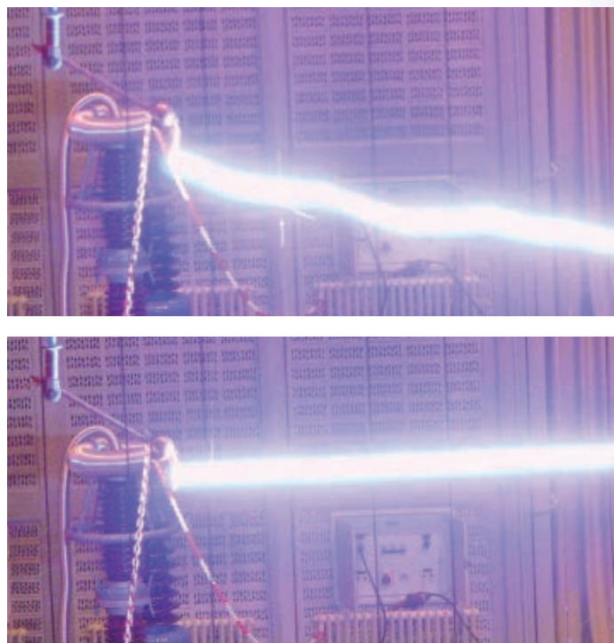
Free (top) and guided (bottom) high-voltage discharges. The high-voltage electrode (spherical, on the left) represents the cloud, while the plane electrode (right) is grounded.
